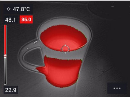
Above alarm : Highlights all pixels with a temperature above the specified temperature level.
